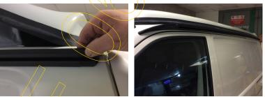
When the front and rear end stops are finally positioned, and you are happy with the appearance, mask off the surrounding area and fill any gaps around the end stops with sealant. Ensure that you clean off any excess sealant using the retained wipe. You can also use white spirits or panel wipe to clean off excess if you have accidentally smudged or over applied sealant. Please allow 24 hours to cure fully before attaching any awning or roof rack etc. Dispose of any unused products responsibly.
